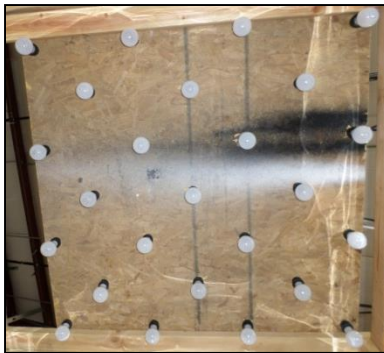
Figure 2.2: Light Bulbs Installed in Light Board
