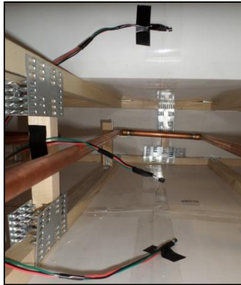
Figure 5.1: Placement of Thermistor Locations Inside the Model Building
